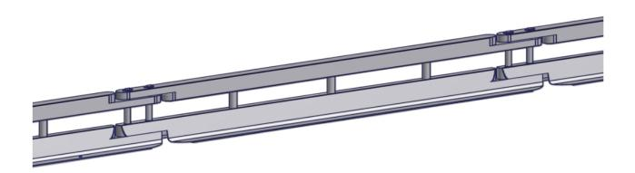
The double-sided vehicle restraint system comprised of galvanised components. The installation length is 20.52 m. The system is characterised by its four wall elements, connected and anchored by insertion posts. The two middle elements are removable and equipped with rollers so that they can be shifted manually.
