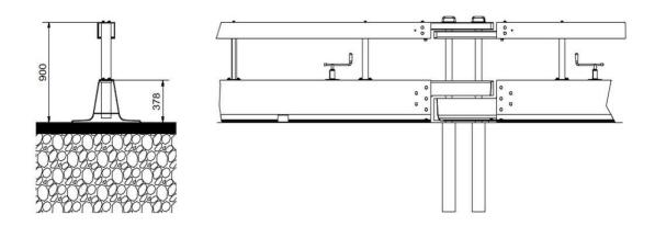
The double-sided vehicle restraint system can be is composed of galvanised components. The installation length is 36,6 m. The system is characterised by its two halves and the opening point in the middle. The system halves are fixed to the ground by two sleeve posts each. The system halves may be seperated from each other after removing the sleeve posts. The halves of the system may be equipped with extractable rollers, so that they can be shifted laterally.
