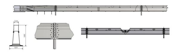
The double-sided vehicle restraint system comprised of galvanised components. The installation length is 36-120 m. The system is characterised by its four wall elements, equipped with hinges. The system is fixed to the ground by sleeve posts and transition elements. The two middle elements are connected to each other by two shiftable bars. The wings of the system are equipped with extractable rollers, so that they can be shifted manually.
